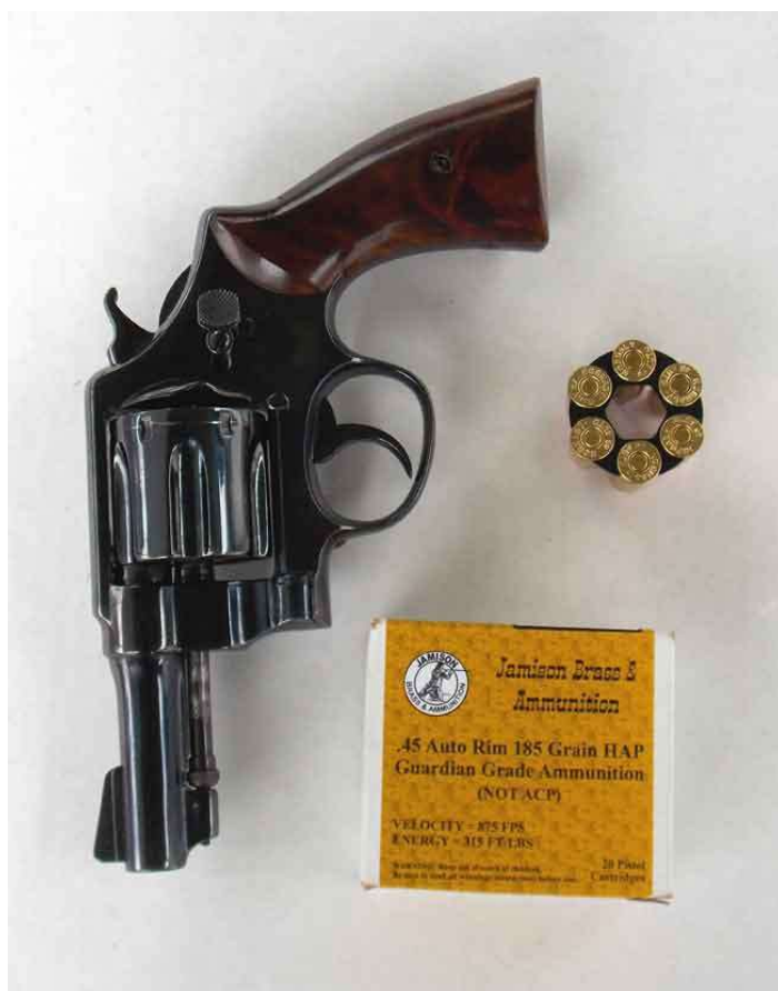
Jamison Brass Captech loads and the Smith & Wesson Model 1917 make a good combination. Note the six-round full moon clip with .45 ACP ammunition.
